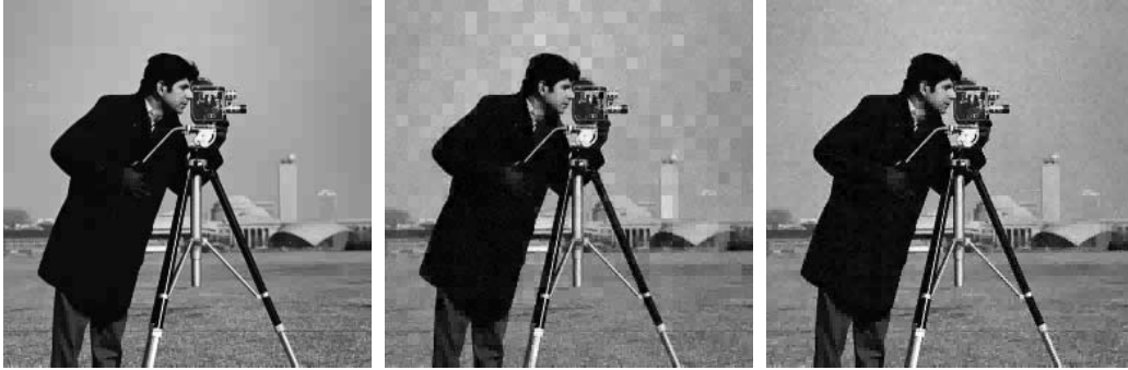
Figure 2. Left: 256 \times 256 pixel natural image with sparsity = 15% in the Haar wavelet domain. Middle: reconstructed image using about 25% data with noiselet. The error is -24 dB. Right: reconstructed image using chirp. The error is -41 dB, much better than that of noiselet.
