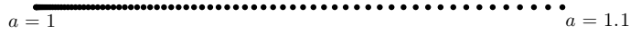
FIG. 3.4. Nonuniform sampling values of a in [1, 1.1] . The spacing between values grows linearly.
