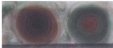
FIGURE 11. An example of the two-celled pattern with a saddle point in the centre of the container. Here, \delta_c = 0.79 , \delta_h = 2.4 , and Re = 2.13 \times 10^4 .
