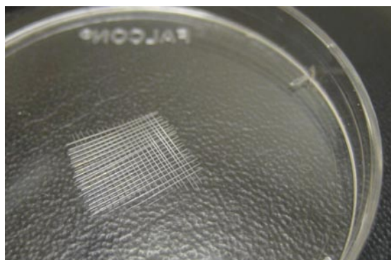
Fig. 13 – Small etchings provide a way to hold the eggs in place without polylysine.
