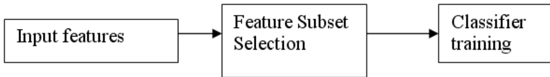
Figure 3: Filter method uses the characteristics of data to select features in preprocessing phase.
