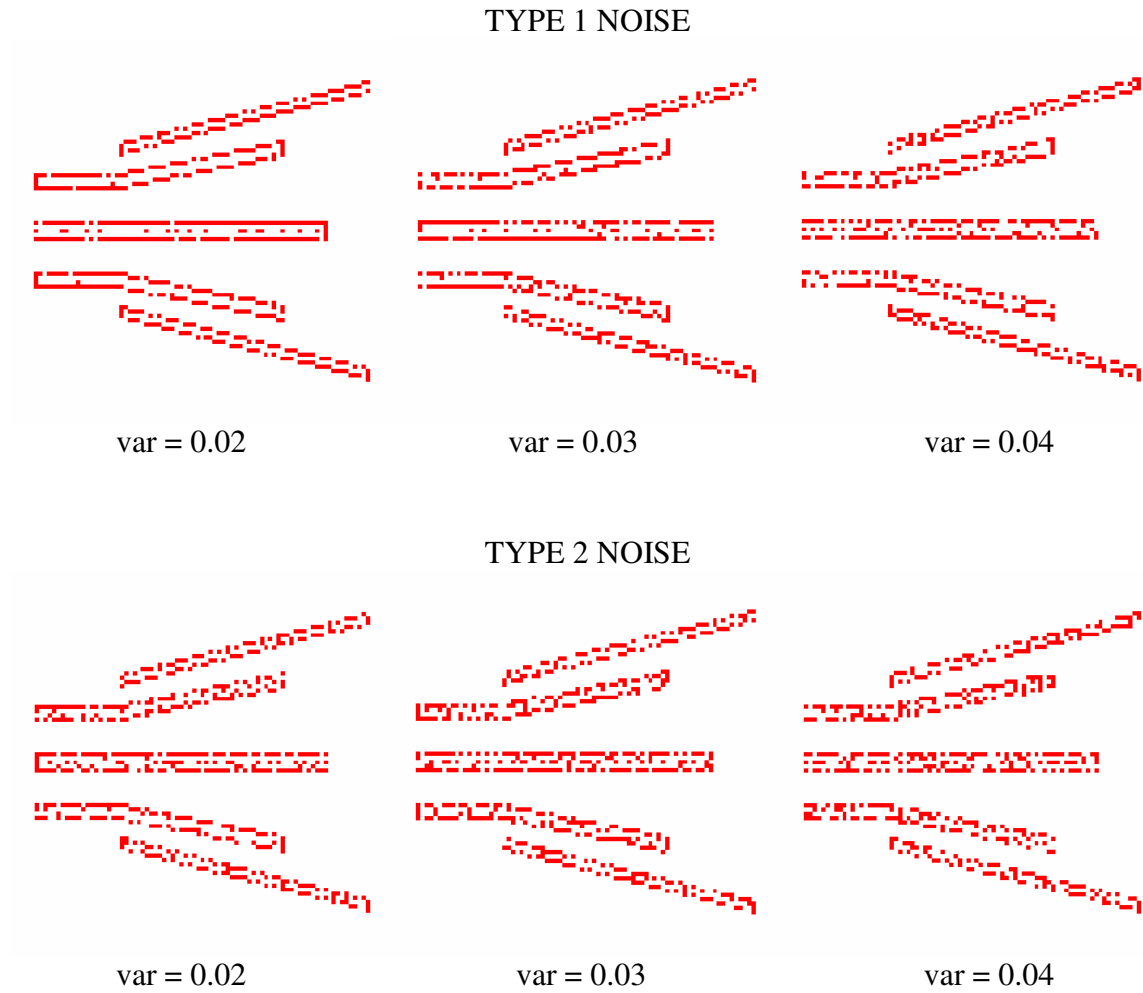
Figure 6 Effects of Type 1 noise where P_{ngn}[0] is a normal distribution with mean = 0.58 and different variance (var). Parameters in Table 1 and C_{notch} = 0.075 were used. Effects of Type 2 noise where P_{ngn}[0] is a normal distribution with mean = 0.58 and var = 0.03 and noise that is normally distributed with mean = 0 and different variance was added to P_{ngn}[t] at each interval. Parameters in Table 1 and C_{notch} = 0.075 were used.
